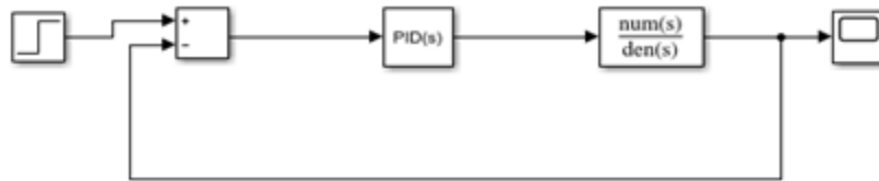
Figure 3.2: The PID configuration for the kiln contro
